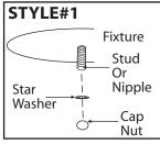
**STYLE#1**- Tuck electrical wires into outlet box and position fixture over studs or nipple on mounting bracket assembly. Secure fixture in place with star washer(s) and cap nut(s). **Note:** If required, assemble body and spread the arms of the fixture out evenly.
