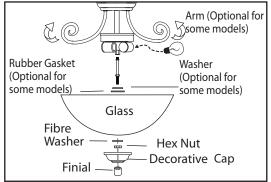
Spread the arms evenly. Attach the stem to the fixture and position the glass over the stem. Secure the glass in place using the fibre washer, hex nut, decorative cap and finial. Install proper bulb type and wattage.
