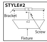
**STYLE #2** - Insert one screw into the mounting bracket - do not tighten yet. Tuck electrical wires into outlet box and position fixture over the mounting bracket. Line up the screw in the bracket to the "7" hole on the fixture. Slide fixture to secure in place. Insert remaining screw. Tighten both screws to secure.
